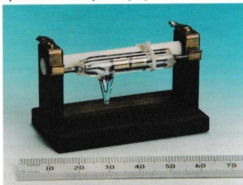
17 The replica coherer used in these investigations
