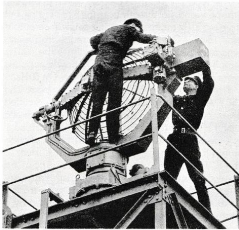
2 The dish antenna of the naval version of a Type 277 radar
