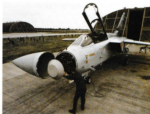
1 Foxhunter radar installed in a Tornado aircraft
