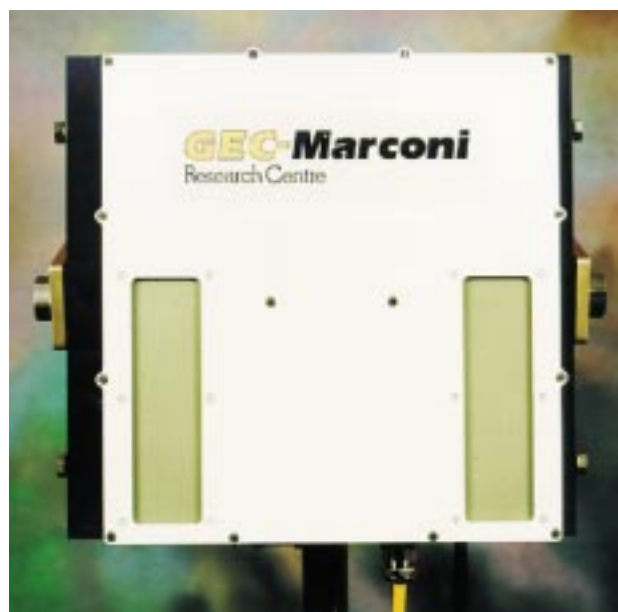
9 Communications unit providing a radio interface to a fibre network
