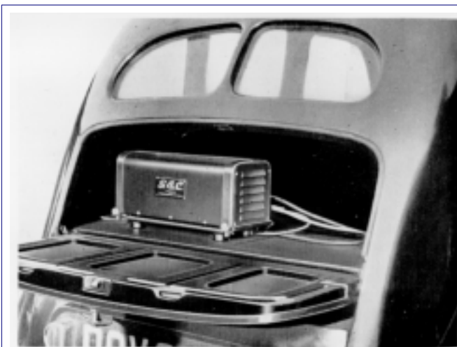
Typical mobile installation showing the transmitter/receiver in the luggage compartment of a car
