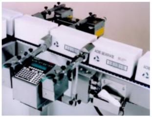
The new Videojet Apollo II Ink Jet Imager with NT Print Controller is a large-character, high resolution carton coding system that excels at printing bar codes, text and graphics onto corrugated containers or similar porous materials. Its high quality performance in this field of application results from the ability to adjust print contrast, as well as from features such as bar code width control, bar code magnification and vertical printing capability.
